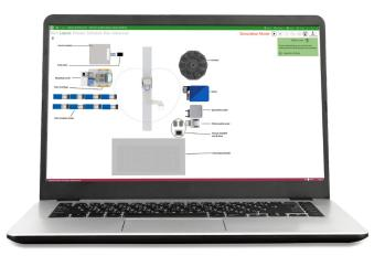
Historically, protein purification has been a manual process involving hand-pipetted samples, vacuum manifolds and other rote, error-prone and timeconsuming tasks. The protein purification workcell system layout in Green Button Go software enables scientists to design and change workflows quickly and run reproducible methods 24/7.
