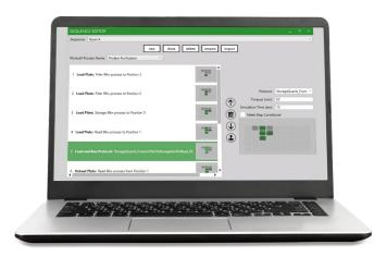
The sequence editor in the liquid handler driver configures complex plate movements. It builds a deck editor to match the liquid handler and establish the order of plate movements for the protocol, minimizing the risk of deadlocks, wasted samples and incomplete or unsuccessful runs.
