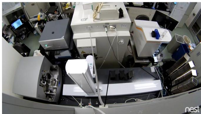
Figure 1. Notable Labs high throughput WorkCell driven by Biosero's Green Button Go software.
